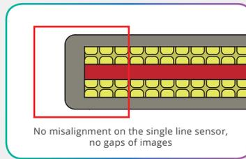
SingleSensor technology provides high-quality scanned image. As a single line sensor covers full width to scan, edge of small texts and thin lines can be sharply and clearly reproduced, without misalignment between sensors.
