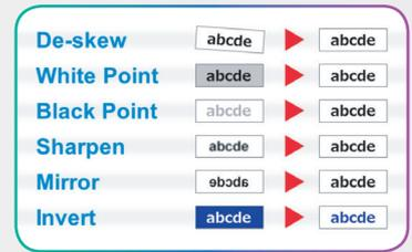
Abundant image enhancement features are incorporated such as de-skew, white point, color reversal of diazo print and restoration of deteriorated original images, which is useful for archiving old drawings.
