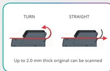
Front entry and rewind to front path (u-turn like), which is often used for regular scanning of plain paper document. Straight path of front entry to rear exit makes it possible to scan documents up to 2.0 mm thick.
