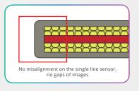
SingleSensor technology provides high-quality scanned image. As a single line sensor covers full width to scan, edge of small texts and thin lines can be sharply and clearly reproduced, without misalignment between sensors.
